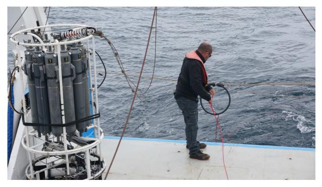
Working from the rear deck of the R/V *Téthys II*: deployment of the Biospherical C-OPS free-fall underwater radiometer, while the CTD Rosette is waiting for subsequent deployment.
